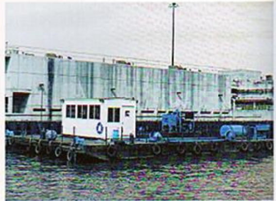
Self-propelled sectional barges utilizing a hydraulic power system, including dual outrives, and a four point Pullmaster winch anchor system.
