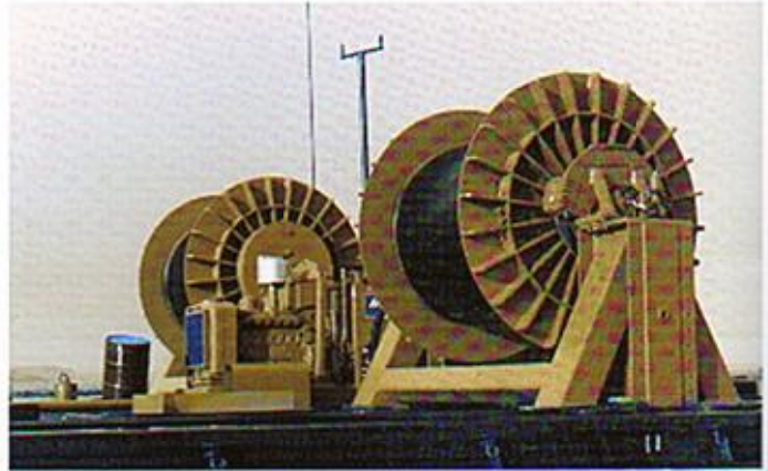
Custom designed, hydraulically powered winches with capability for spooling 3" wire rope.
