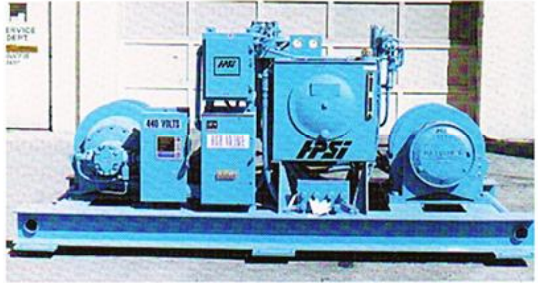
Electric over hydraulic two drum barge mover.
